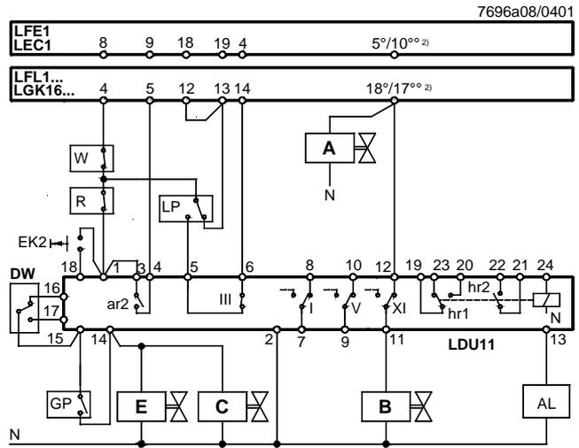
**Valve proving test with 2 pressure switches**
