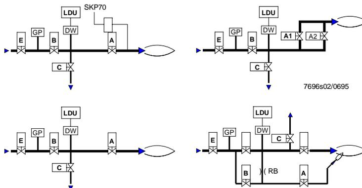
**Connection examples without vent pipe to atmosphere (for applications not covered by EN 676) using burner controls LFE..., LFL... or LGK..., or the control unit LEC...**
