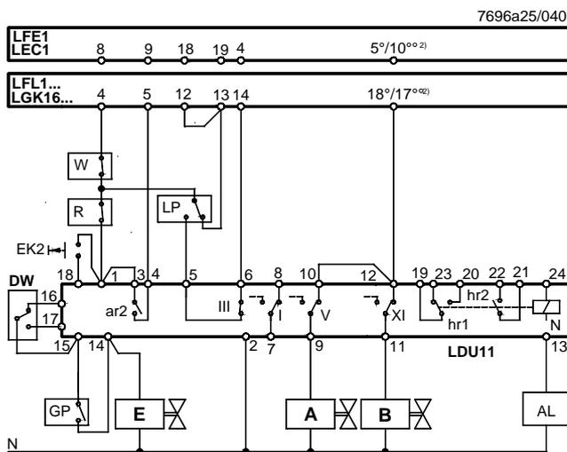
Valve proving test with 2 pressure switches
