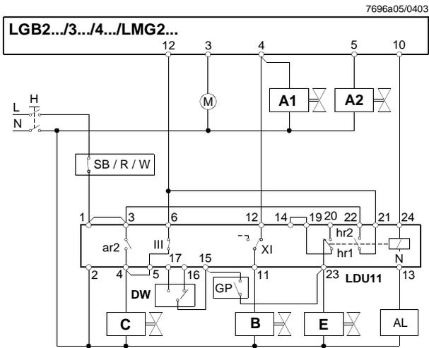
Valve proving test following immediately the controlled shutdown
