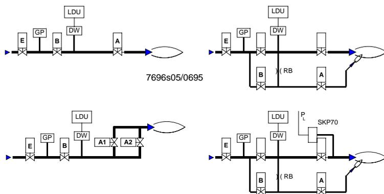
**Connection examples without vent pipe to atmosphere using burner controls type LFE..., LFL... or LGK..., or control unit LEC... and the SKP70... with expanding flame burners**
