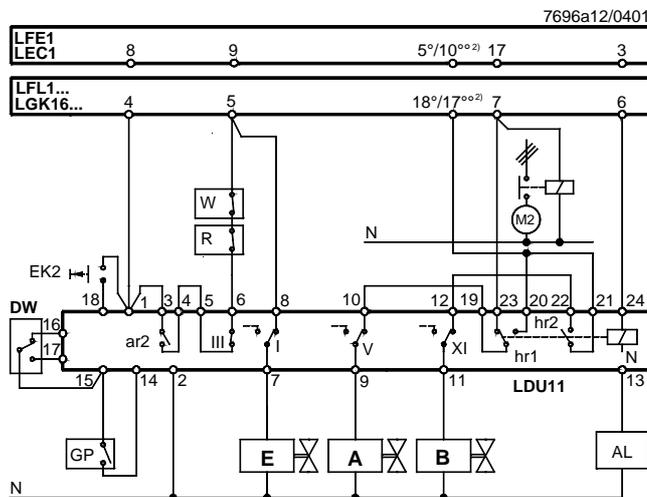
**Valve proving test with 2 pressure switches**
