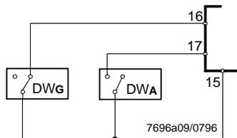
Air pressure «PL» for the SKP... must be sufficiently high to open the SKP70... although the burner's air damper is closed.
