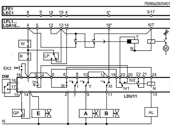
Valve proving test during the prepurge time (min. 60 s)
