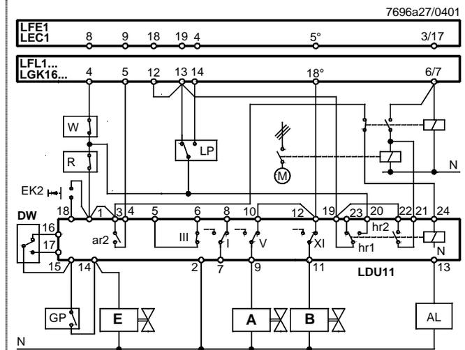
Valve proving test with 2 pressure switches
