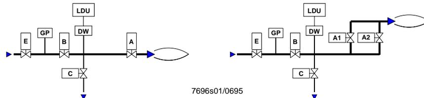
**Connection examples with vent pipe to atmosphere using burner controls type LFE..., LFL... or LGK..., or the control unit LEC...**
