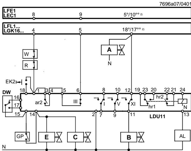
Valve proving test during the prepurge time (min. 60 s)
