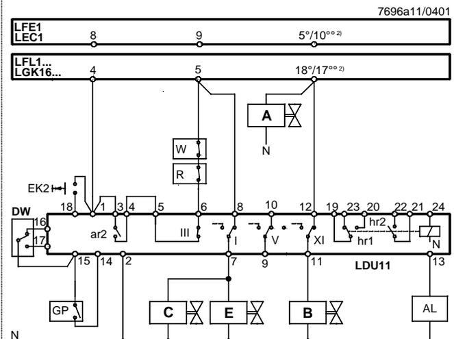
**Connection examples with vent pipe to atmosphere using burner controls type LFE..., LFL... or LGK..., or the control unit LEC...**
